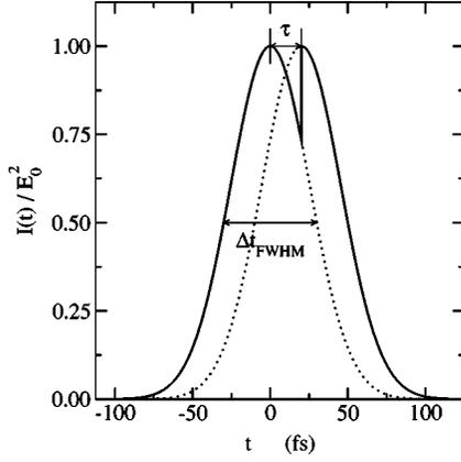
FIG. 1. Time-dependent normalized intensity resulting from two time-delayed ( $\tau=20$  fs) identical, linearly polarized Gaussian femtosecond ( $t_{\text{FWHM}}=60$  fs) laser pulses (parallel configuration) neglecting the time overlap of the pulses.
